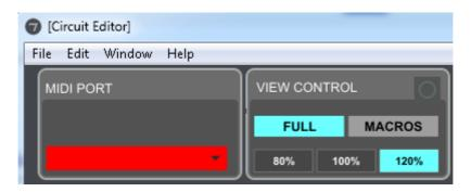
If the MIDI Port looks like the image above. You *are not* connected! (Make sure you are in the standard mode and *not* the bootloader)
