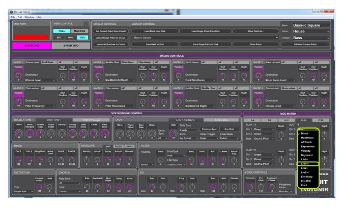
In this example I am selecting **Lfo1** +/- **in Mod Matrix slot 14**, **source 1**. This will feed the **Lfo** output to **Source slot 1**.
